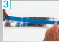
Find the halfway point of the blue straping that you have cut so equal amounts will hang over each end and stick it on the sticky tape on the
