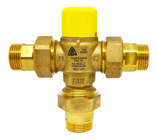
The tempering valve is designed to keep the outlet conditions of the mixed water stable, even if the inlet conditions vary. In hot water production systems with storage, so as not to accelerate development and growth of legionella, the hot water must be stored at a temperature of at least 60°C; at this temperature the bacteria can neither survive nor reproduce.
