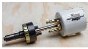
Once the gold pins on the adapter meet the arbor, turn the gold quick release knob on the top of the arbor clockwise to lock the arbor to the adapter.
