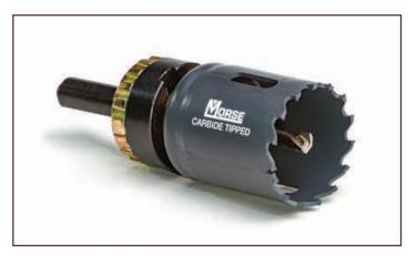
Long lasting choice for very hard abrasive materials. These materials too hard or too abrasive for standard bi-metal holesaws, or so thin they would strip bi-metal or chip carbide teeth. Cutting depth of 1-1/2". Arbor required.
