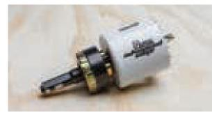
Using a fast adapter, screw clockwise in to top thread of the holesaw until finger tight.
