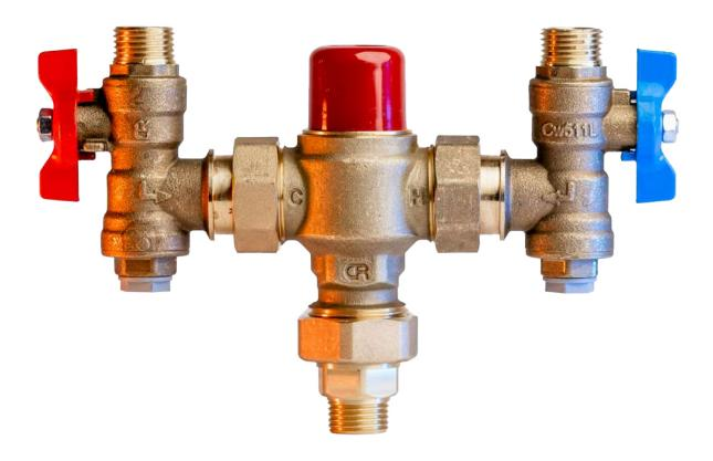
The RBM thermostatic mixer valve for solar systems is designed to keep the outlet conditions of the mixed water stable, even if the inlet conditions vary. In hot water production systems with solar storage, the temperature of the water in the storage tank can vary greatly depending on radiation and on the amount required by the users.
