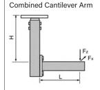
Combined Cantilever Arm from Beam Section TP F 80 1 x End Support WBD-F 80 1 x Cantilever Bracket AK F 80 8 x Self-forming Screw FLS F 80
