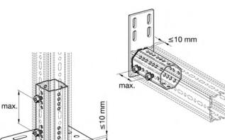
Assembly to Beam Section TP F 80, for instance Cantilever Bracket AK F 80 and others.
