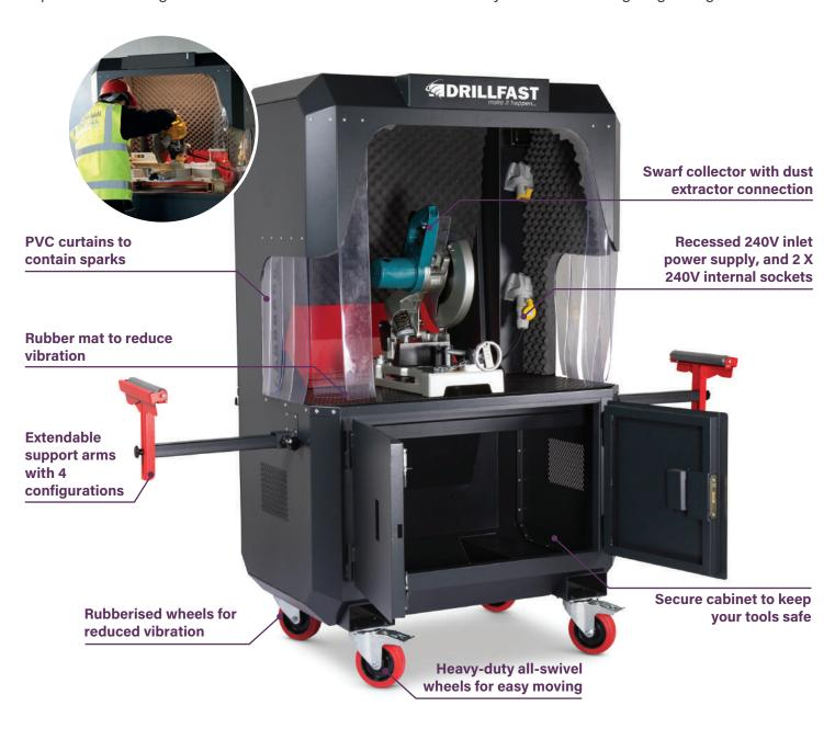
CodeWeightExternal Dimensions W x D x H (mm)Internal Dimensions W x D x H (mm)30ASS7175kgStandard 1390 x 750 x 1900 Extended 1390 x 1070 x 1900Top (with extended back) 1140 x 1020 x 960 Bottom 1135 x 710 x 550
